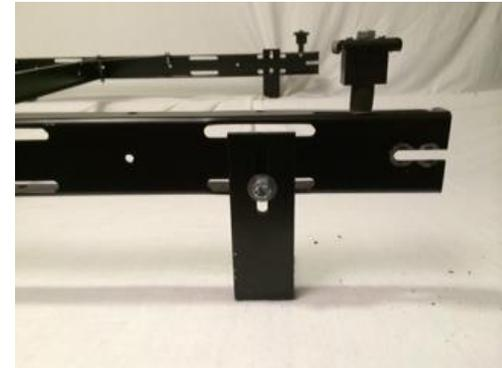
The placement of the feet allow for multiple positions that are preset based upon 16",24", and 48" spacing of roof rafters, the feet can be easily adjusted if from position to position, but in most cases width adjustment to match roof rafters will not be needed.
