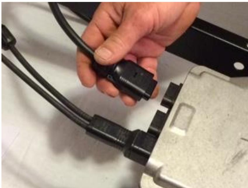
Connect the inverter cables to the inverters per the inverter instruction manuals for proper connections
