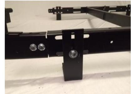
The anchor feet also allow for vertical adjust to compensate for variances in roof levels, while maintaining minimum height distance from roof to the bottom of the solar panel
